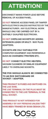
Should a power column be fitted, the cover of the power column should only be removed by a qualified electrician, and only once the power source has been isolated. The inside of the power column is a live electrical installation, in accordance with BS 7671: 2008. A warning label appears on the access panel, as shown here.
