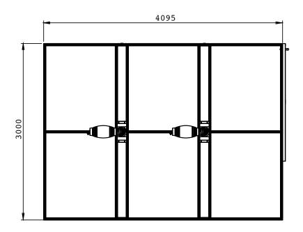
Standard height: 2275mm External height with airflow unit: 2430mm
